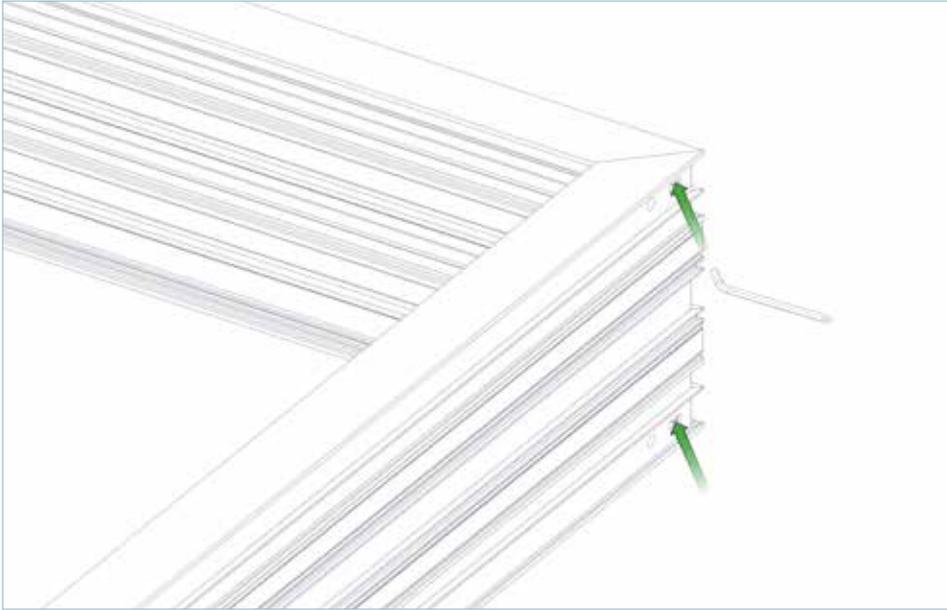
Tighten the cleat join with a 4mm Allen Key and screws provided.
