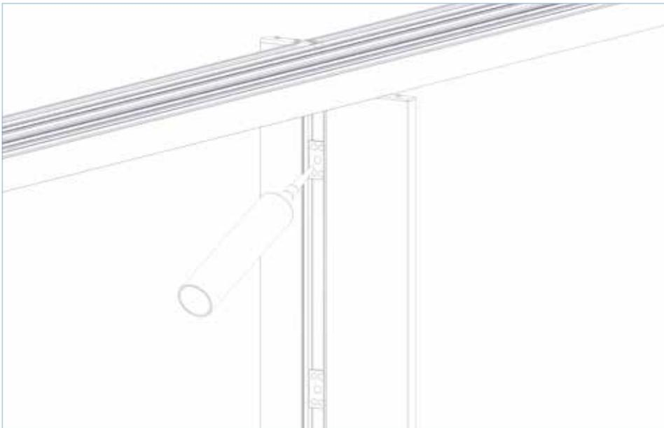
Apply supplied structural sealant around each packer.
