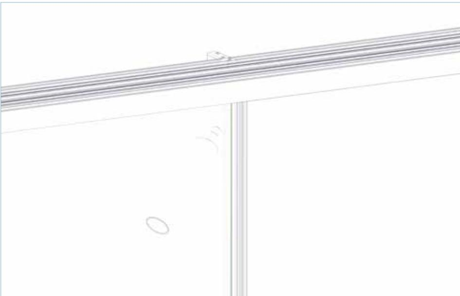
Apply bead of structural sealant along the length of interlocker (both inside and outside faces). Leave to fully cure before operating the set.
