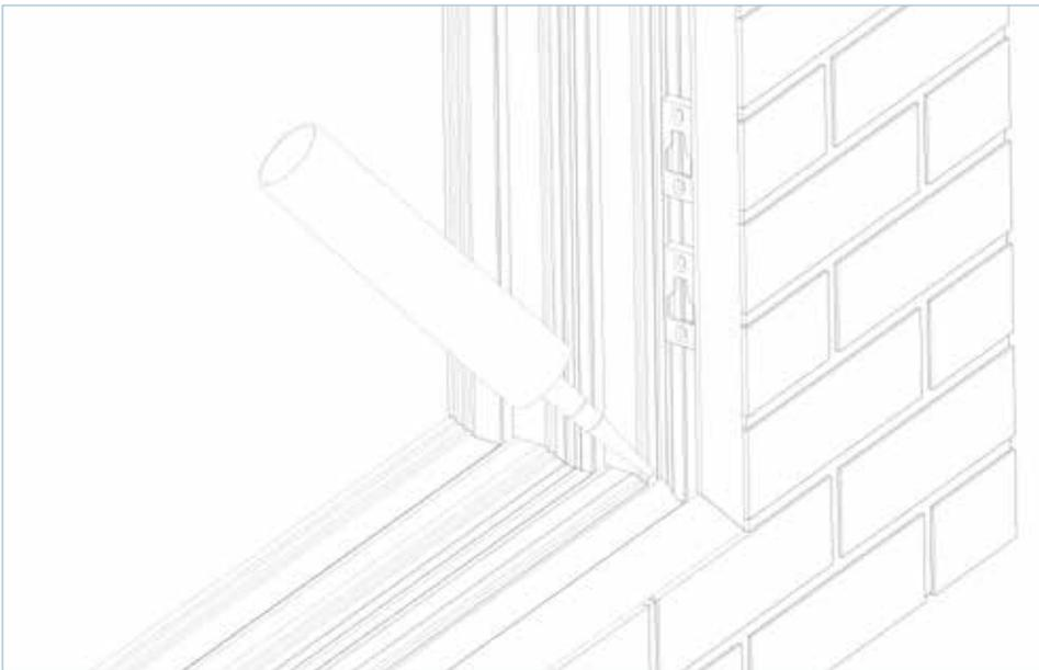
Seal the drainage isolator in place, ensuring ends of profile are sealed with edge of frame.
