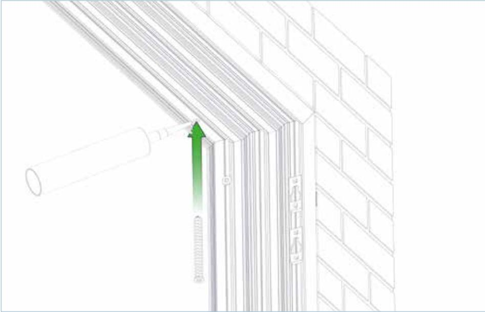
Insert suitable sealant to fixing hole, then screw preferred fixing in place. This must be done at both ends of the top track.
