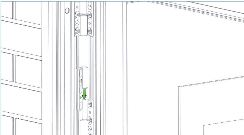
16. Find the separately provided hinge leaf and slide onto the exposed hinge pin.
