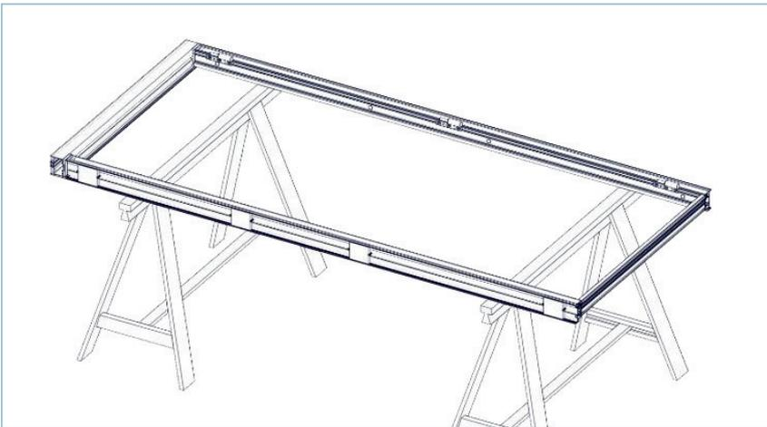
9. The outer frame should now be assembled and secured together.
